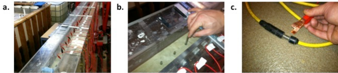
Figure 5.2 (a-c). (a) Photo of the electrode spacing (approximately 6.25 cm) along a surface profile (b) Close-up photo of the electrodes being inserted directly into the soil surface (c) Photo showing electrical components used to connect electrodes to main ERT data cables.
